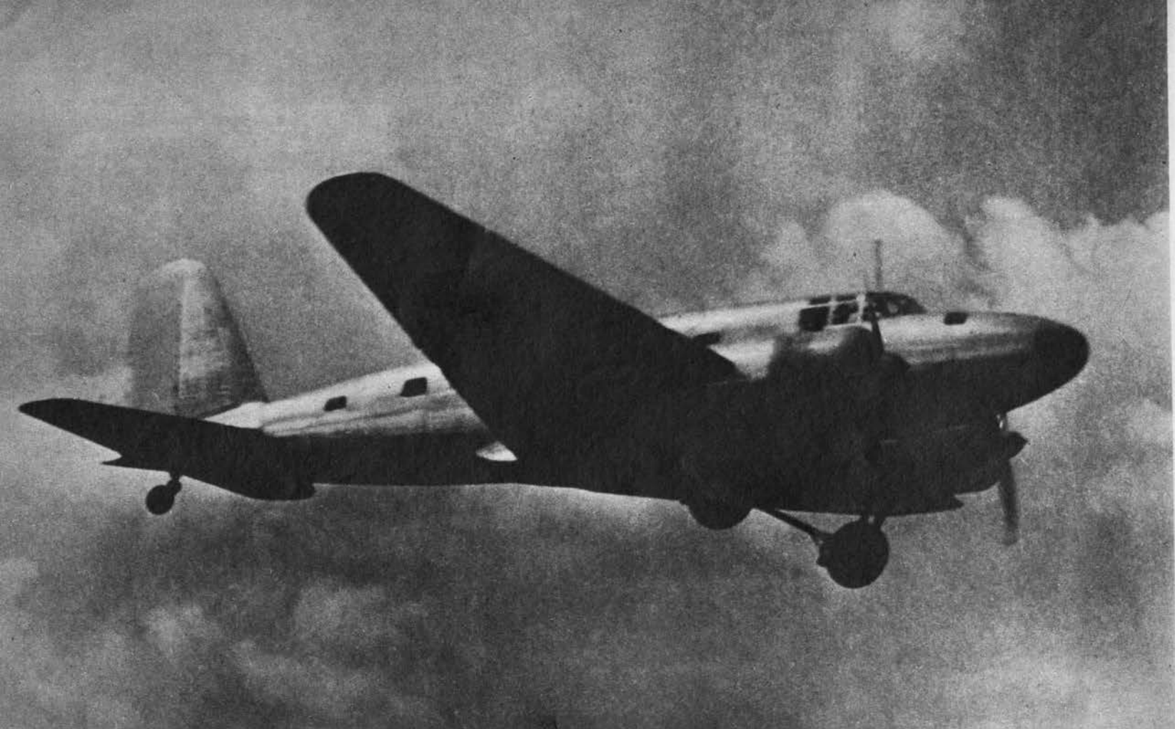
TOPSY, CHIEF JAP ARMY TRANSPORT, HAS A LONGER NOSE, MORE SLENDER FUSELAGE THAN U.S. TYPES. BOTH WING EDGES TAPER EVENLY
